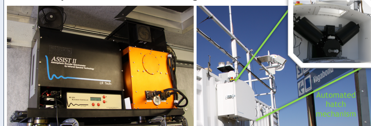
Figure 3. ASSIST (left) deployed inside the ARM Mobile Facility 2 (right) at the Mount Werner site (Colorado) in support of STORMVEX [2]. The instrument performs measurements 24/7 unless rain or snow are present, in which case the automated hatch mechanism (insert) is closed to protect the equipment. Courtesy of Pacific Northwest National Laboratory
